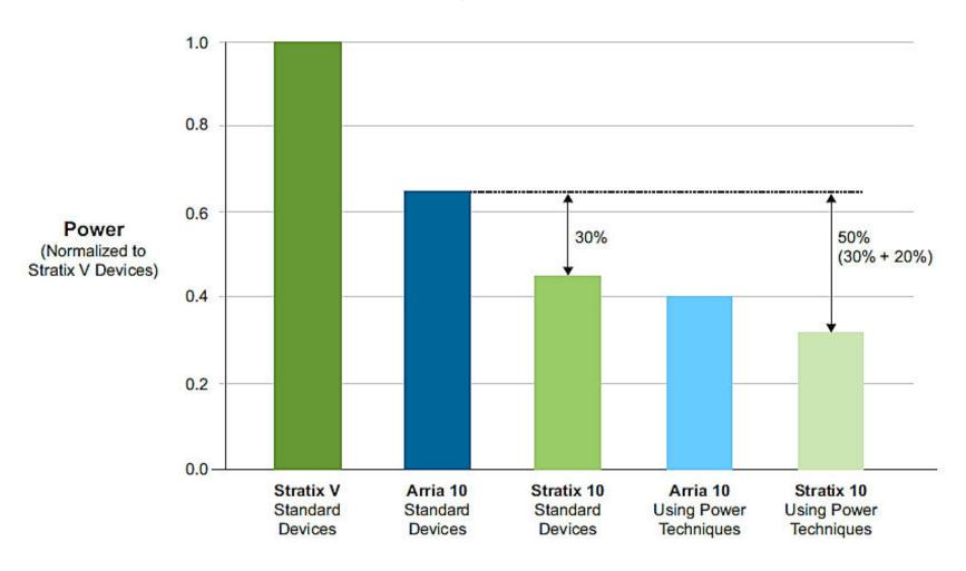
Significant power reduction expected in Altera ® Stratix 10 FPGAs
