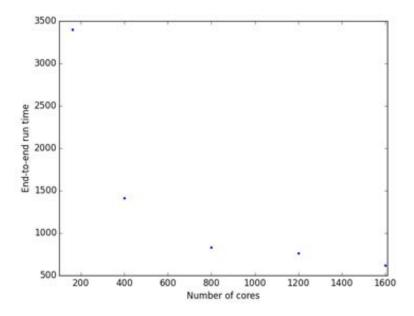
Scaling with number of cloud cores used. Includes calculation of uncertainty and collation and combination of data. Download of the result adds roughly 10 seconds.
