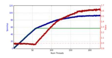
Speedup as a function of number of threads. Ratio shows the speedup over the number of physical cores – it should be 1 until hyper-threading starts.
