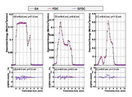
Dose distribution projected into each plane. Differences between Geant4 and the GPU track repeating implementation are around 2 %
